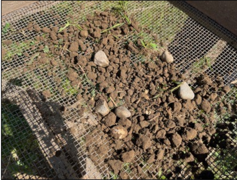
Image 9: Representative image showing gravel fills within disturbed test pit.
