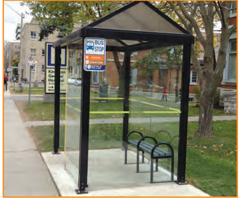
Example of accessible shelter, dimensions 1,524 mm x 2,348 mm (5 ft x 8 ft) with minimum entrance of 1,117 mm (44 in).
