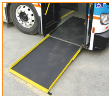
Ramp with contrasting colour strips and slip-resistant surface.
