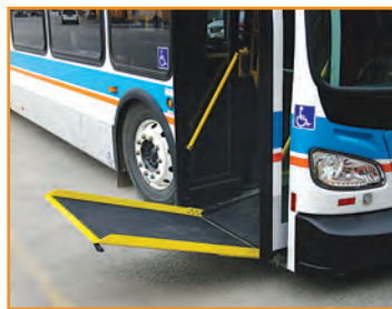
Bus ramp being lowered.
