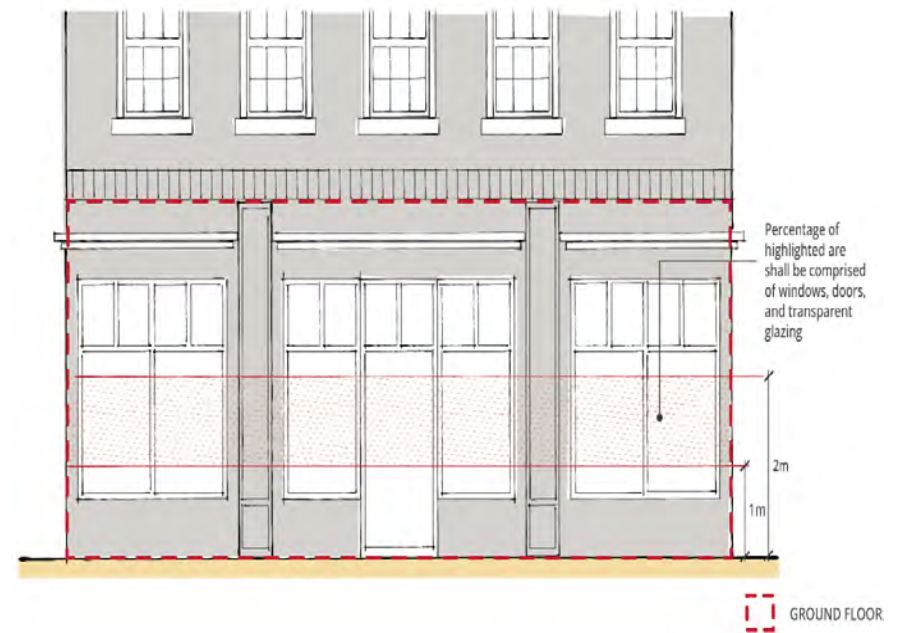
FIGURE 5.7.3. Ground Floor Treatment between 1.0m – 2.0m
