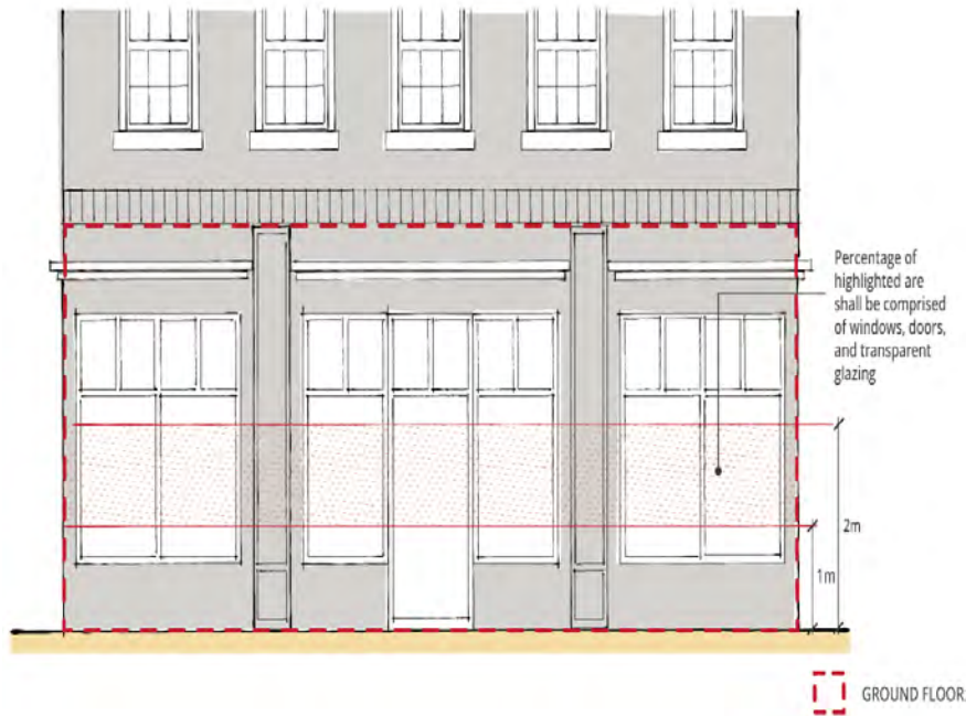
FIGURE 5.6.2. Ground Floor Treatment between 1.0m – 2.0m
