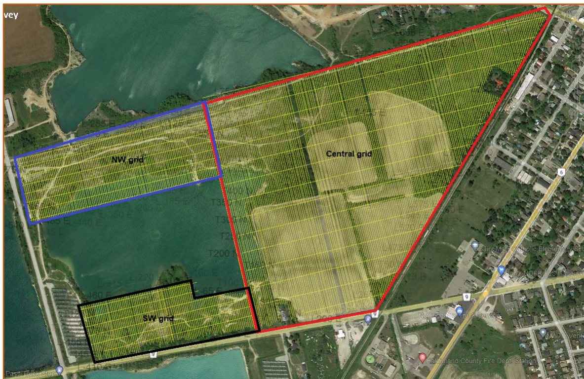
Figure 3. Drone magnetic flight coverage over the Sandusk Residential Development (SRD) Project.
