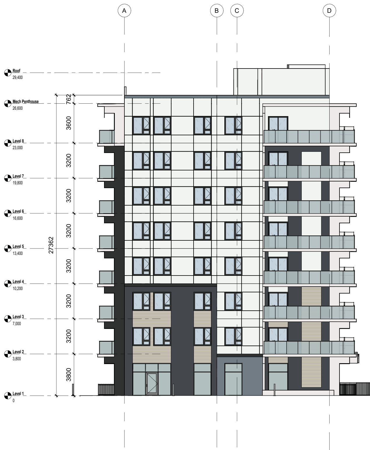
2 BUILDING ELEVATION NORTH 1 : 200 .A.400.
